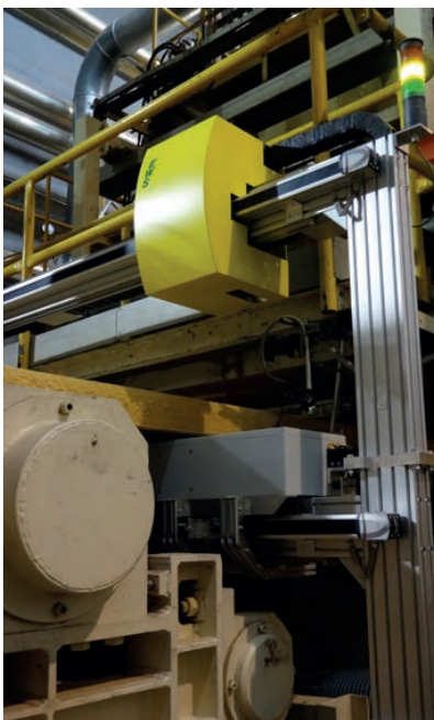
Above left: Figure 2 – Traversing area weight gauge MASS-SCAN X ME with MultiEnergy technology for various measuring tasks in panel production
